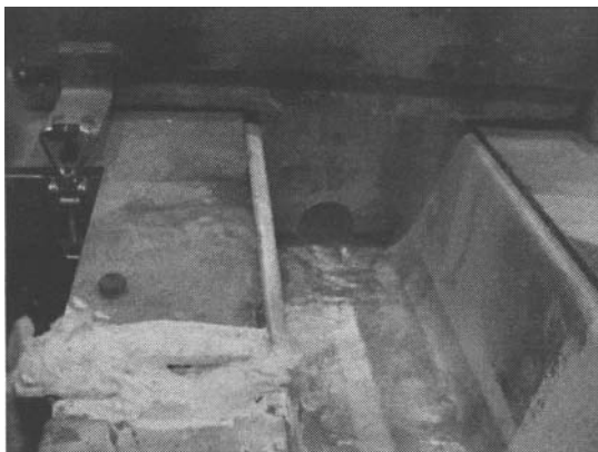
Figure 11. View of the exit flow from the cyclone showing that the exit flow tube is only partially filled.
