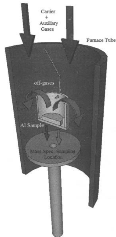
Figure 3. Diagram of the sample within furnace tube.
