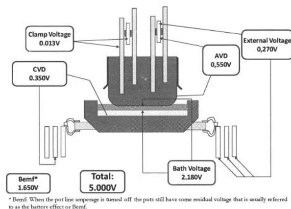
Fig. 1 – Break up of total pot voltage (typical).
