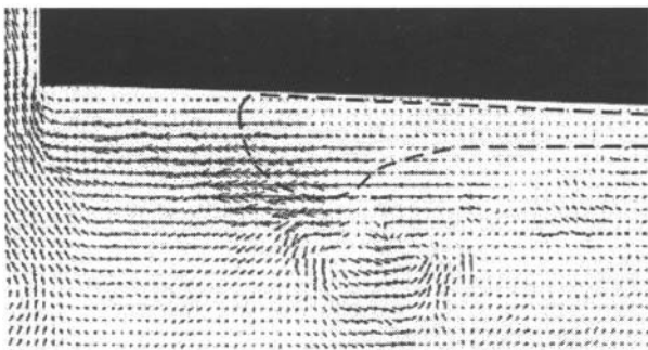
Figure 4. Instantaneous velocity field around a Fortin bubble
