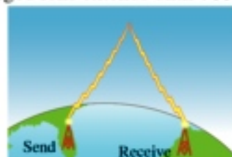
Reflection of radio waves from the ionosphere Figure (13)
