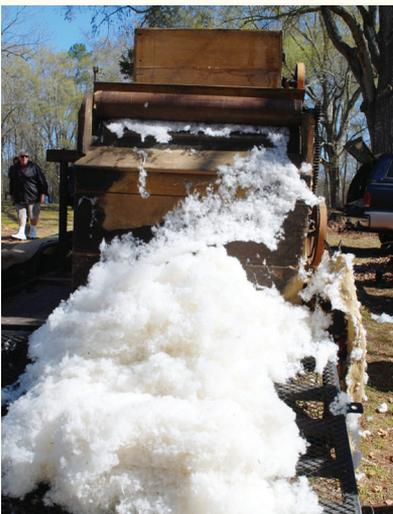
The first step to turn cotton into cloth is to separate it from the seeds. There is a machine that can help. The machine is called a cotton gin .
