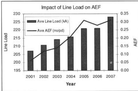
Figure 6. Impact of Line Load increase on AEF.
