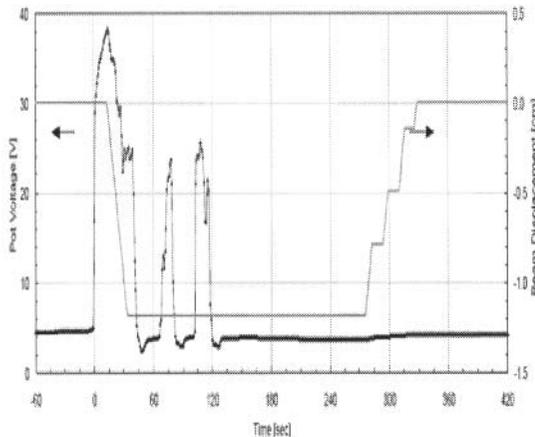
Figure 3. The rapid rise in voltage following the onset of an anode effect
