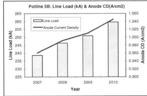
Figure 11. Line Load vs Anode Current Density
