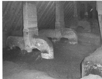
Figure 9. Uniform Anode Top Ore Cover
