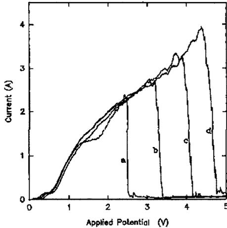
Figure 2: Potentiodynamic voltammogram of a carbon anode electrolysed in cryolitic electrolyte. (a)=0.75 wt%  $\text{Al}_2\text{O}_3$ , (b)=1.75 wt%  $\text{Al}_2\text{O}_3$ , (c)=2.75 wt%  $\text{Al}_2\text{O}_3$ , (d)=4.55wt%  $\text{Al}_2\text{O}_3$ . From Haverkamp [6]
