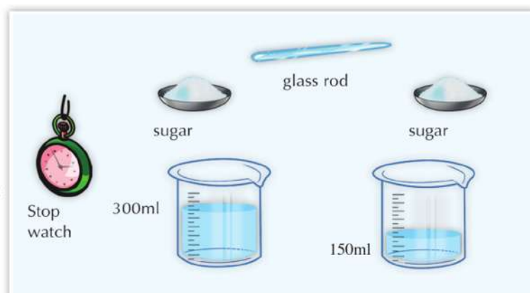
Fig. (41) Increasing quantity of solvent decreases dissolving time.
