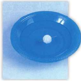
fig. (21) A piece of cork, with a magnetic needle, floats on water surface.
