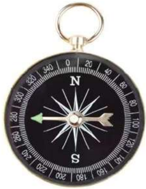
fig. (20) The compass contains a small, light, free moving magnet.
