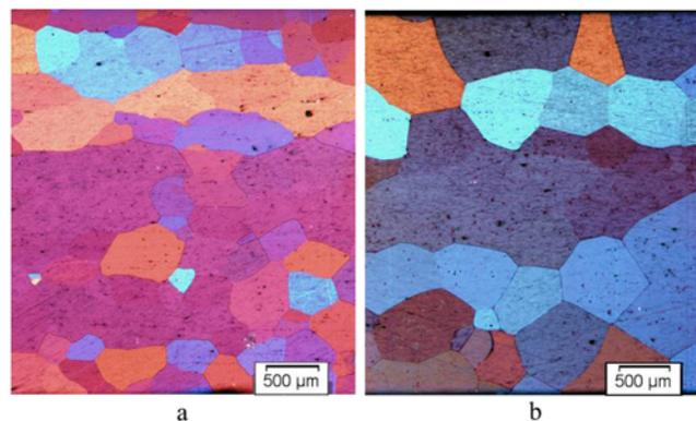
Figure 8. Grain microstructure of the aluminum substrate after 30 min (a) and 140 min (b) soaking at 650  $^{\circ}\text{C}$ .
