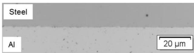
Figure 5. Microstructure of the seam and the parent material of the twin-roll cast clad strip.
