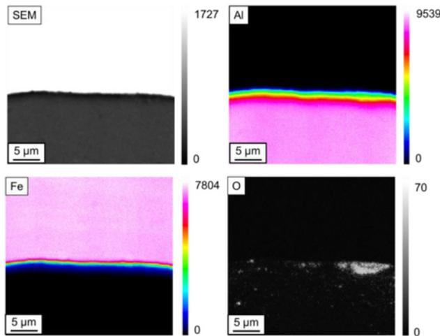
Figure 11. Distribution of the chemical elements in the seam of the hot roll-bonded clad strip (using EPMA measuring counts).
