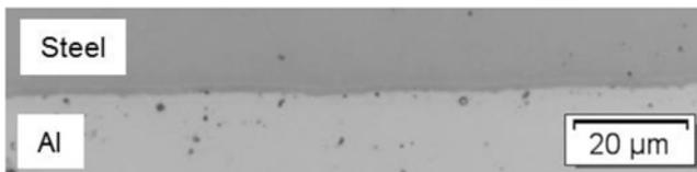
Figure 10. Microstructure of the seam and the parent material of the hot roll-bonded clad strip.
