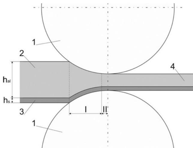
Figure 3. Basic schematic of the roll bonding of aluminum-steel clad strips: 1 –rolls, 2 – aluminum substrate, 3 – steel substrate, 4 – clad strip;  $h_{al}$  – initial thickness of aluminum substrate,  $h_s$  – initial thickness of steel substrate.
