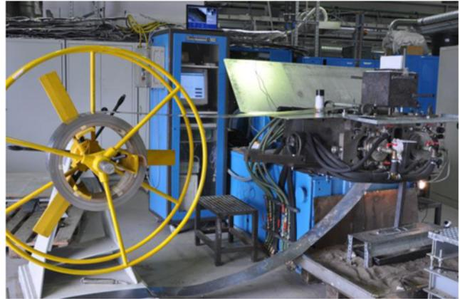
Figure 1. Twin-roll caster used for the clad strips manufacturing.
