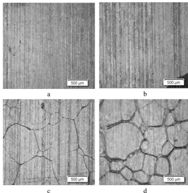
Figure 7. Surface of the aluminum substrates after holding in furnace at 650  $^{\circ}\text{C}$  without protective atmosphere for: 0 min (a), 30 min (b), 140 min (c), 225 min (d).
