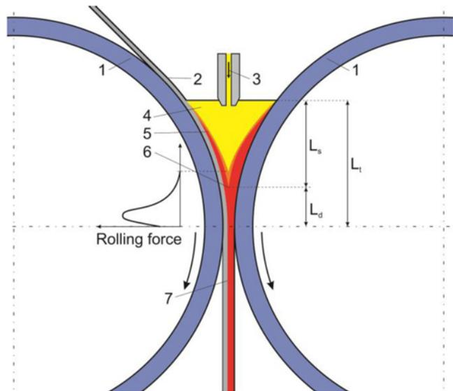
Figure 2. Basic schematic of the twin-roll casting of aluminum-steel clad strips: 1 – water-cooled rolls sleeves, 2 – steel strip, 3 – melt feeding system, 4 – aluminum melt, 5 – semi-solid metal, 6 – kissing point, 7 – clad strip;  $L_s$  – solidification zone length,  $L_d$  – deformation zone length,  $L_t$  – total length of the strip formation zone.
