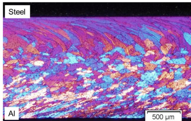
Figure 4. Grain microstructure of the aluminum layer of the twin-roll cast clad strip.
