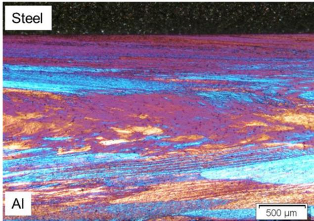
Figure 9. Grain microstructure of the aluminum layer of the hot roll-bonded clad strip.
