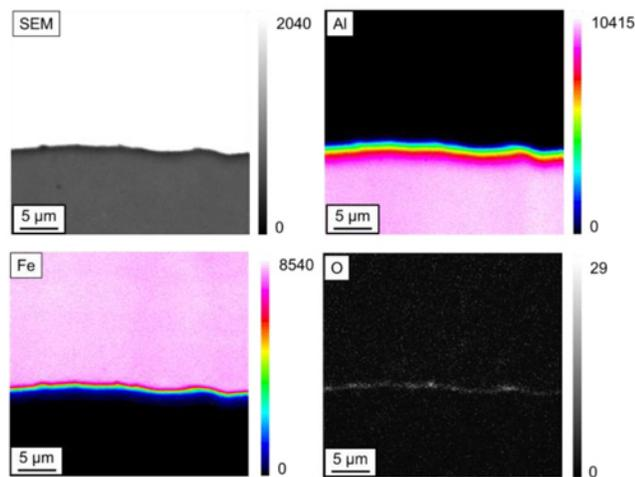
Figure 6. Distribution of the chemical elements in the seam of twin-roll cast strip (using EPMA measuring counts).
