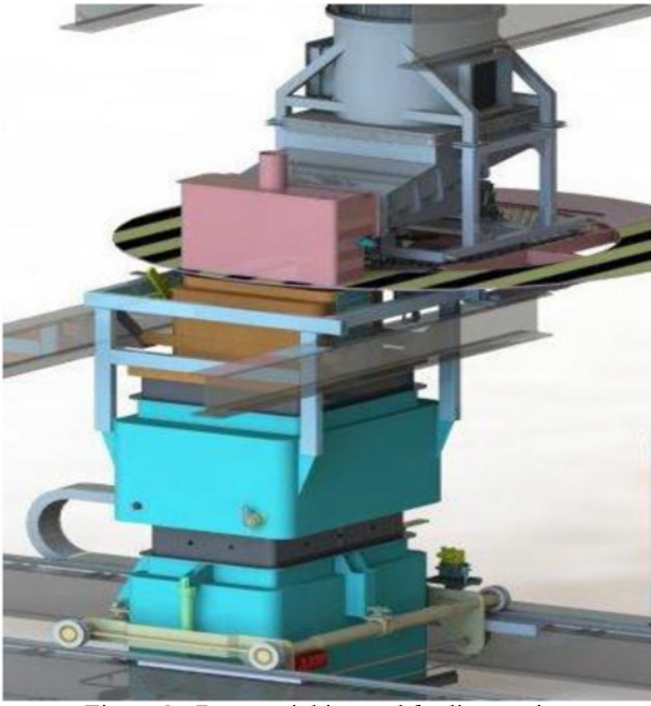
Figure 8 - Paste weighing and feeding equipment
