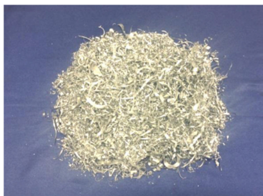
Figure 1 Machining chips of aluminum alloy 380.
