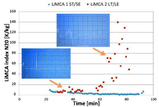
**Figure 15:** Illustration of a LiMCA measurement performed with long electrodes failing after about 30 min of use
