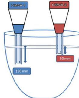
**Figure 10:** Configuration ST/SE (-50 mm) vs LT/LE (-150 mm)
