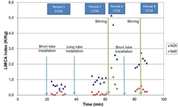
**Figure 5:** LiMCA results obtained in a lab scale crucible (20 kg) – Successive configurations: ST/SE and LT/SE
