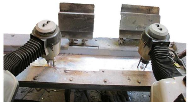
**Figure 16:** Evaluation of in-depth LiMCA measurement in flowing melt
