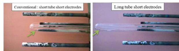
**Figure 2:** Illustration of both tubes combined with short electrodes (sampling hole is indicated by an arrow)
