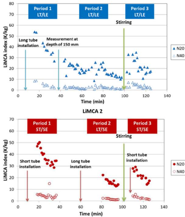
**Figure 7:** LiMCA results obtained in a lab scale trial with 2 LiMCA in various configurations
