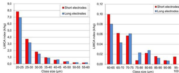
**Figure 14:** Period 2 – Comparison of the histograms obtained when measuring 150 mm under the surface (LiMCA LT/LE and LiMCA 2 LT/SE)
