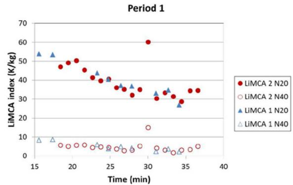
**Figure 9:** Period 1 – Measurement at 50 mm depth with LiMCA 1 (LT/LE) and LiMCA 2 (ST/SE)
