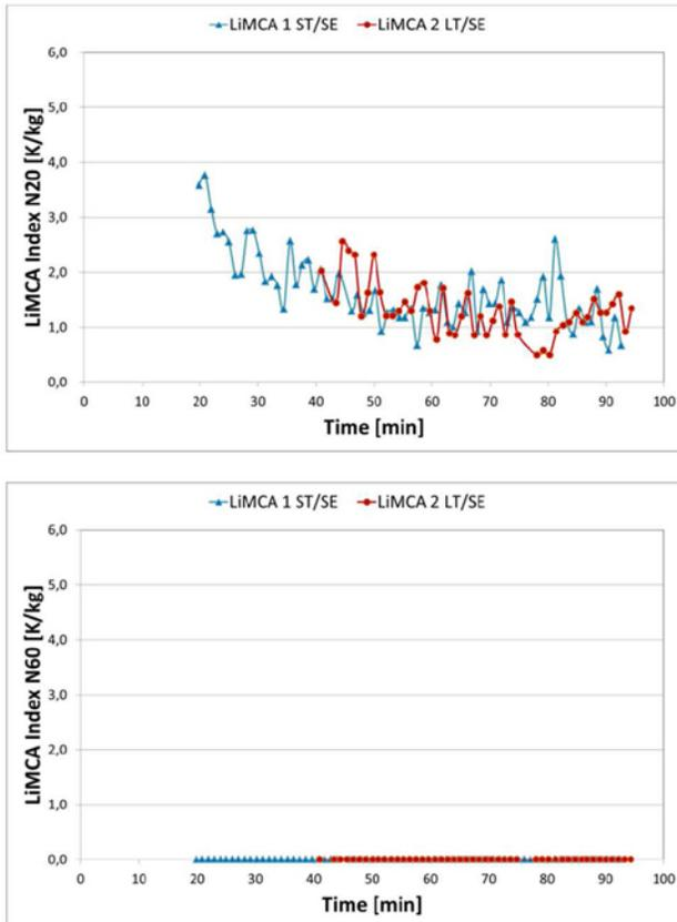
**Figure 17:** Comparison of LiMCA N20 measurements in a trough (casting furnace exit) with short electrodes and long or short tube.
