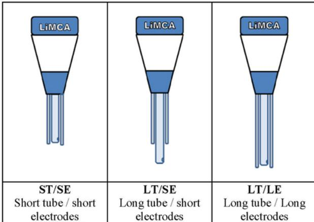
**Figure 4:** Schematics of the three configurations under study
