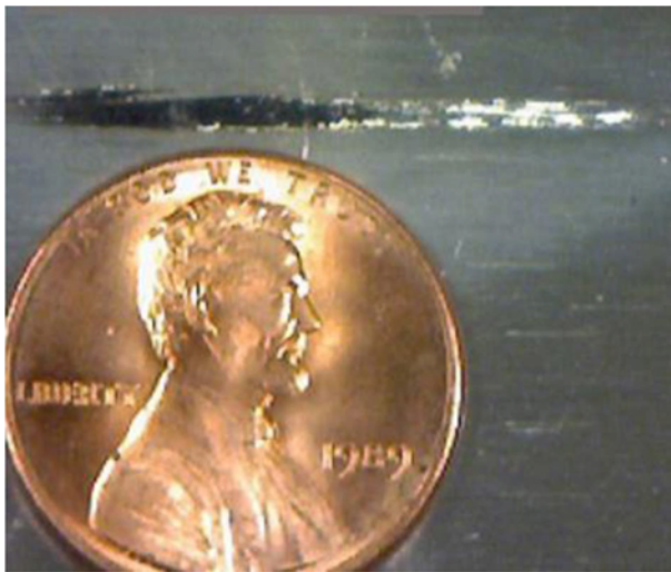
Figure 2: Typical Grade "C" Black Mark
