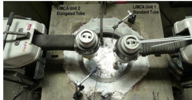
Figure 4. Laboratory test setup using two LiMCA units with LiMCA tubes in different lengths in a 180 kg resistance heated crucible furnace at RWTH Aachen
