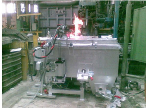
Figure 7. The prototype “OptiFilter” filtration unit under pre heat at Trimet Aluminium.
