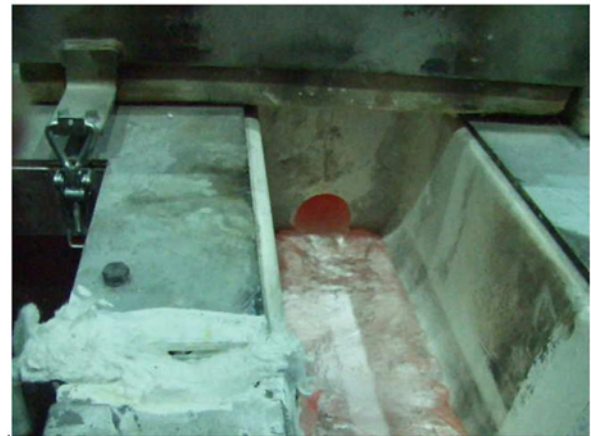
Figure 8. View of the exit flow from the cyclone showing that the exit flow tube is only partially filled.
