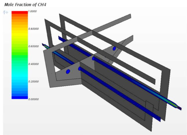
Fig 10: Mole Fraction of CH4 (Open fire Burner)
