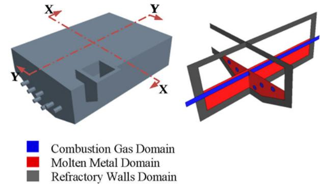
Fig 2: Domains of the Immersed Heater Furnace
