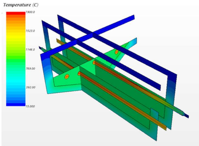
Fig 11: Temperature Profile (Open fire Burner)
