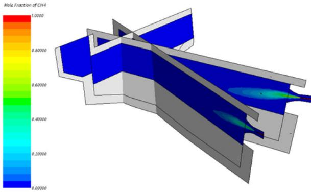
Fig 7: Mole Fraction of CH4 (Open fire Burner)
