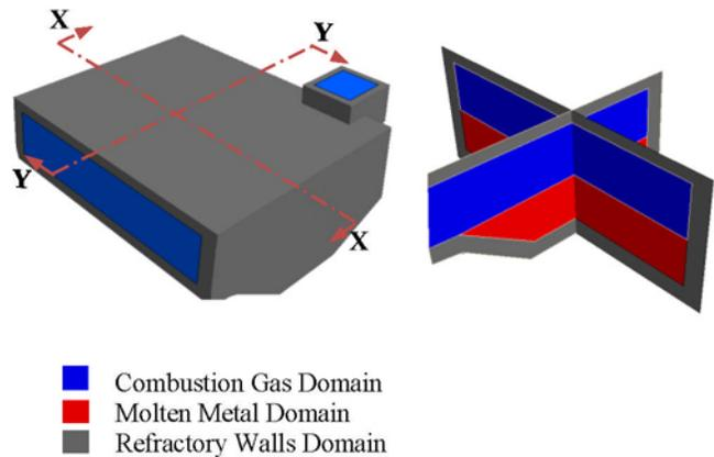
Fig 1: Domains of the Open fire Furnace
