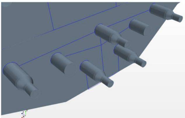
Fig 4: Immersion heater burner
