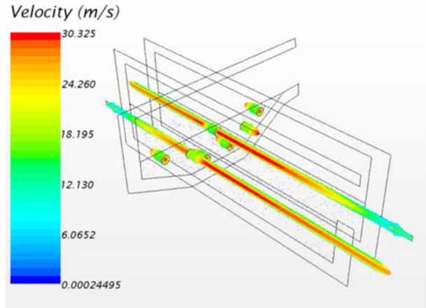
Fig 9: Velocity Profile (Open fire Burner)
