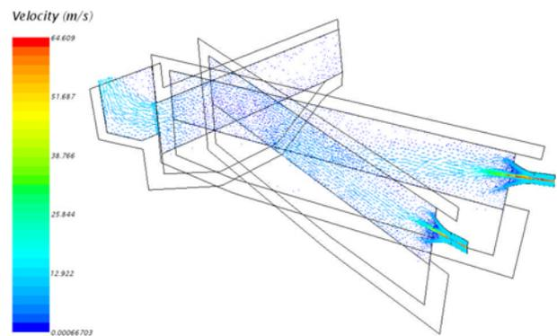
Fig 6: Velocity Profile (Open fire Burner)
