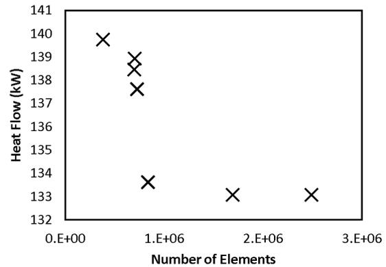
Fig 5: Mesh Sensitivity Analysis
