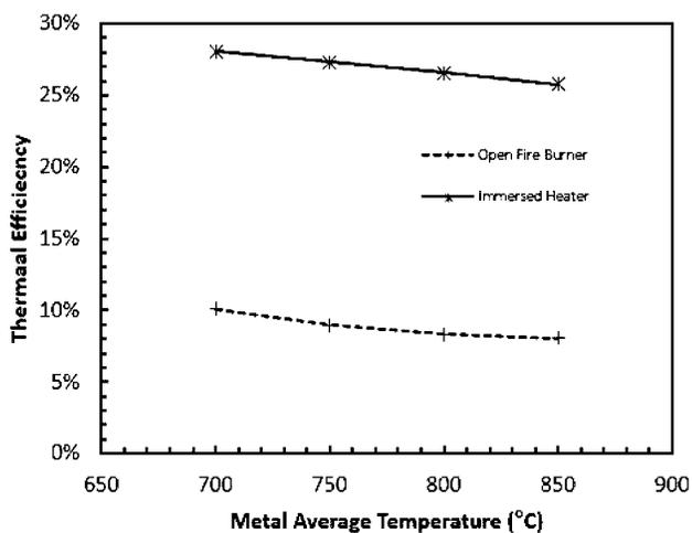
Fig 12: Thermal Efficiency comparison between the open fire and immersion heater.
