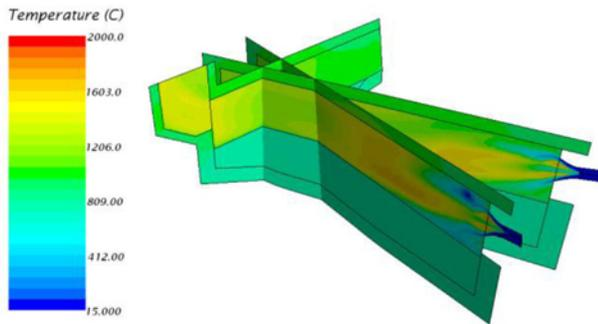
Fig 8: Temperature Profile (Open fire Burner)
