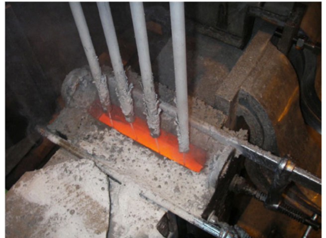
Figure 9: The ESW joint after removing the retaining shoes but before cutting and polishing showing the solidified slag
