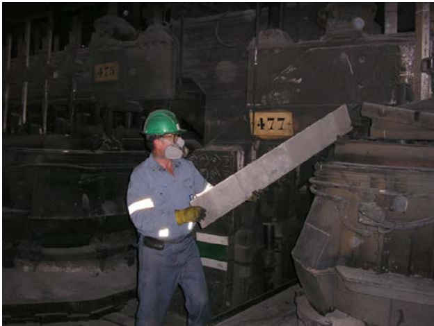
Figure 7. Aluminum plates were added to the top of anodes to form slots in VS Söderberg anodes at Aviles.
