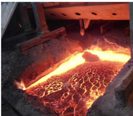
Figure 7: The result of the clean cavity using PTM pacman
