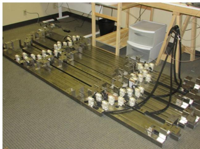
Fig. 1 Slaves, insulated and fixed to rectangular tubing for mounting underneath the anode bus (shown upside down before shipment from WIT)
