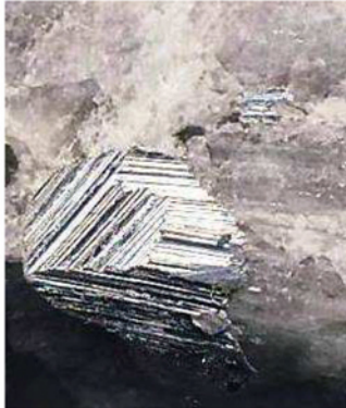
Figure 2. Aluminum droplets enclosed in the side-ledge taken at the metal level
