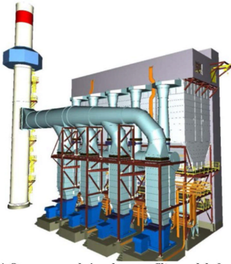
Figure 4. Ozeos: an eco-designed process filter module for GTCs
