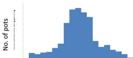
Figure 5: Statistical distribution showing frequency of pots at maximum noise during AE quenching at Nordural.
