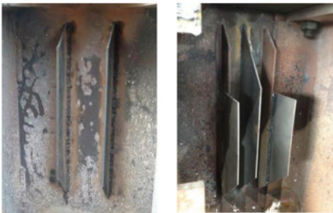
Figure 14: Original double and new D18 sidewall cooling fins.
