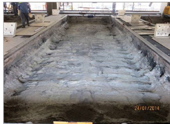
Figure 16. Cathode block surface topography and side lining.
