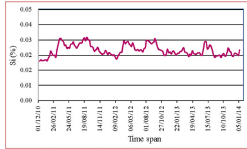
Figure 9. Si percentage in the metal.
