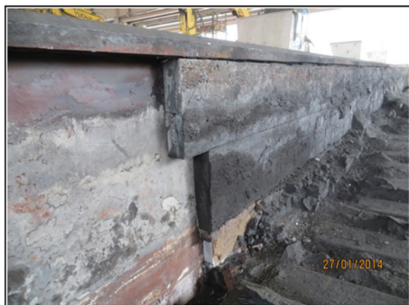
Figure 18. DX+ Sidewall SiC blocks and potshell.
