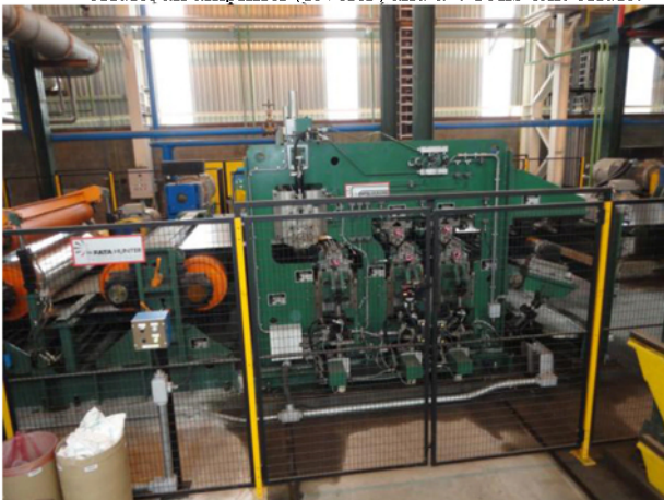
Figure 4. Tension Leveler of the Coil Coating Line.
