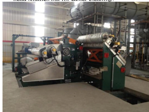
Figure 12. View of the Coater Head on the Coil Coating Line.
