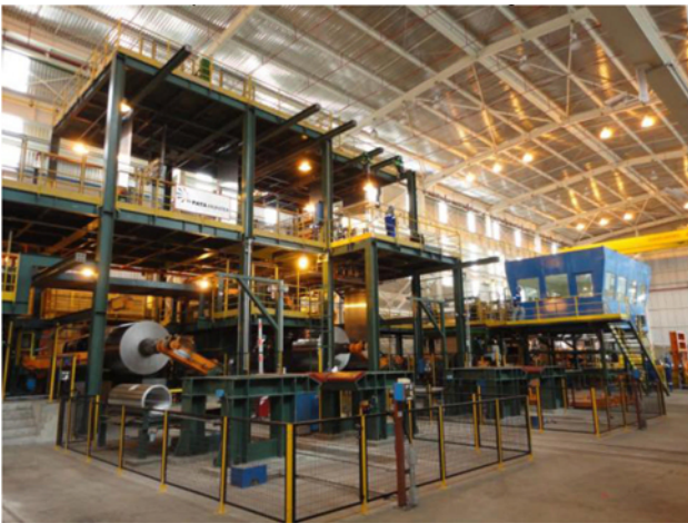
Figure 3. Entry Section of the Coil Coating Line.
