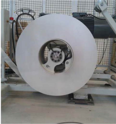
Figure 6. A 200mm wide aluminium coil ready for testing at Lindes DFI pilot plant lab in Stockholm.
