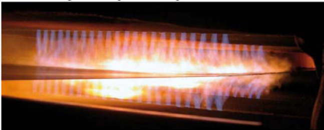
Figure 3. In the photo, four oxy-fuel burner rows are seen directly firing onto a steel strip.
