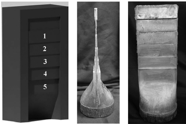
Figure 1 a) 3-D model of step casting mold, and b) side view and c) front view of 5-step casting sample of Al 7075 by squeeze casting under an applied pressure of 60MPa.
