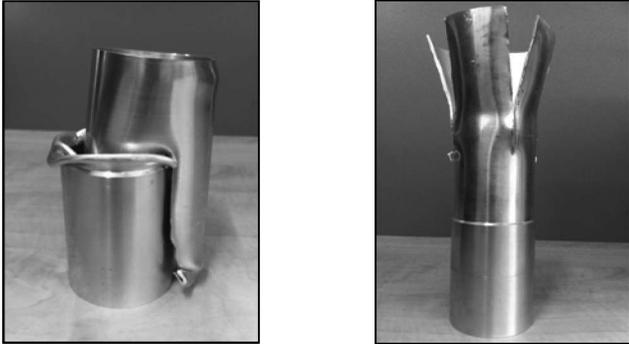
Figure 3: Aluminum extrusions subjected to quasi-static crushing (a) and cutting (b) post test.
