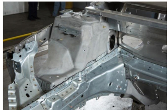
Figure 8. MMLV aluminum shock tower casting joined to the front end assembly by SPR and CMT methods
