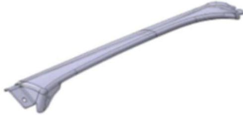
Figure 3. Solid model of the A-pillar cover (~650 mm overall component length).
