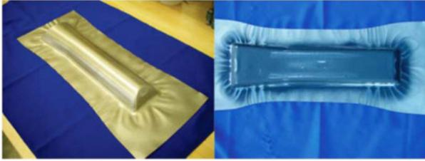
Figure 2. Bottom view of hot formed tray (left) and final formed tray (right) showing sheet draw-in around the perimeter.
