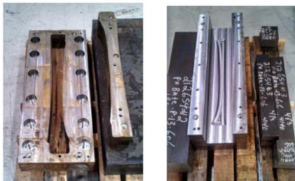
Figure 4. Views of forming tools used to fabricate A-pillar covers.
