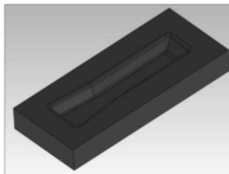
Figure 1. Three-dimensional prototype tray component die design.
