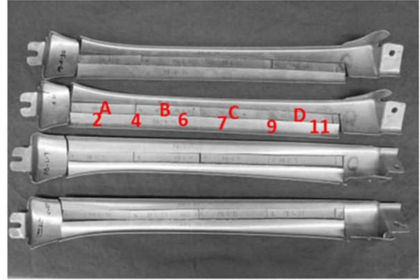
Figure 5. Photograph of several A-pillar covers with cut sections showing the locations where the tensile coupons were obtained from along a cover's length.
