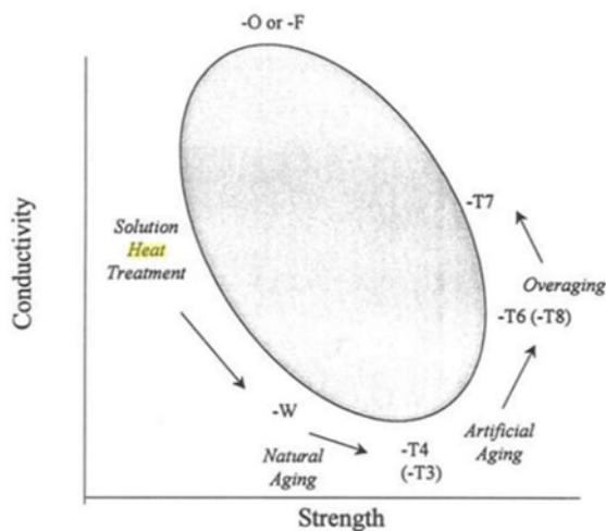
Figure 9. Changes in electrical conductivity and strength with heat treatment [5].
