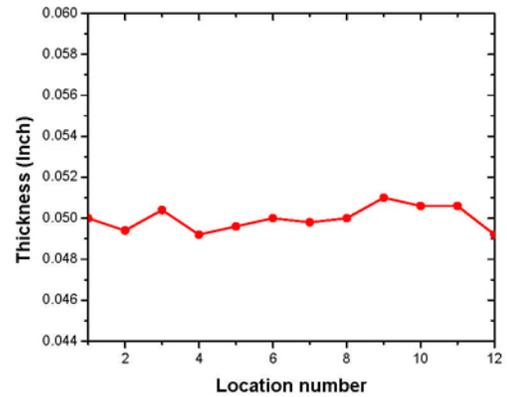
Figure 6. Sheet thickness, measured with an ultrasound gauge, along the length of an A-pillar cover. (0.050" = ~1.27 mm).
