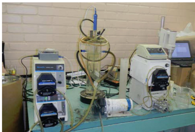
Figure 1. Picture of bench-scale test unit of SUPAFLO thickener
