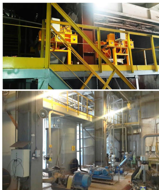
Figure 4. Pilot unit to produce scandium concentrate from red mud.
