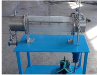
Figure 2. Photo of the self-stirring reactor driven by pressure energy
