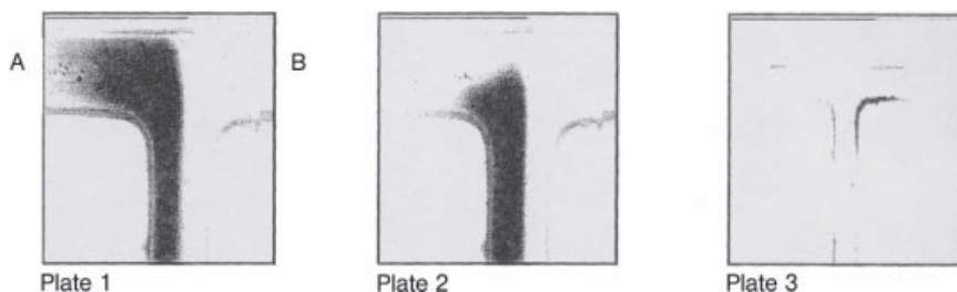
Figure 4.88 Flow patterns, visualized by formation of the colored glide intermediate, allowing one to judge on mixing efficiency [13].
