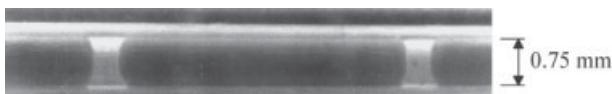
Figure 4.51 Liquid/liquid two-phase plug-flow with plugs of nitrating agent (dark) and organic phase (white) in a capillary micro reactor [94].
