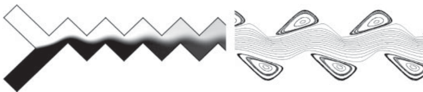
Figure 2.40 Zigzag micro mixer with concentration field (left) and flow stream lines (right) obtained from a CFD simulation for a Reynolds number of 38. In [135] a sawtooth geometry of larger amplitude was considered and distinctive recirculation zones were found only at Reynolds numbers larger than 80.
