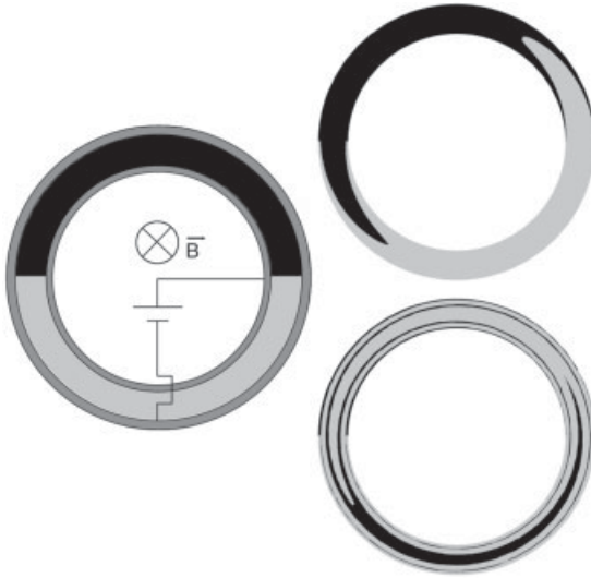
Figure 2.49 The left side shows the schematic design of an annular magneto-hydrodynamic mixer. On the right, the evolution of the interface between two liquids, as described in [147], is depicted.
