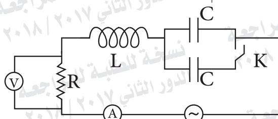
**23- In the circuit shown in figure the phase angle between total voltage ( $V$ ) and current ( $I$ ) passing through the circuit is :**
