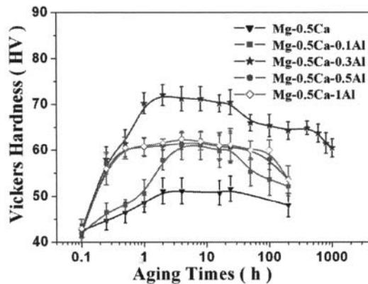
Figure 1 Age hardening response of Mg-0.5Ca-xAl ( $x = 0.1, 0.3, 0.5, 1$ , wt. %) alloys during isothermal aging at 200 °C. Reproduced from reference [8].
