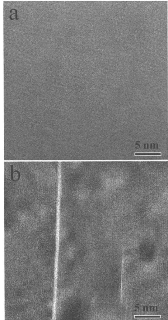
Figure 6 HAADF images of the Mg-0.5Ca-0.3Al aged alloy taken from the  $[10\bar{1}0]$  (a) Peak aged at 200 °C for 2h (b) Over aged at 200 °C for 1000h.
