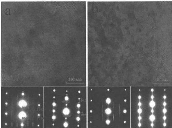
Figure 5 TEM bright field images of the Mg-0.5Ca-0.3Al aged alloy taken from the  $[10\bar{1}0]$  and corresponding SAED pattern of the  $[10\bar{1}0]$  and  $[11\bar{2}0]$  directions. (a) Peak aged at 200 °C for 2h (b) Over aged at 200 °C for 1000h. The figure is reproduced from [8].
