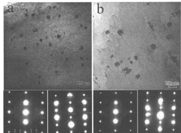
Figure 3 TEM bright field images of the Mg-0.5Ca-0.1Al aged alloy taken from the  $[10\bar{1}0]$  and corresponding SAED pattern of the  $[10\bar{1}0]$  and  $[11\bar{2}0]$  directions. (a) Peak aged at 200 °C for 4h (b) Over aged at 200 °C for 200h.
