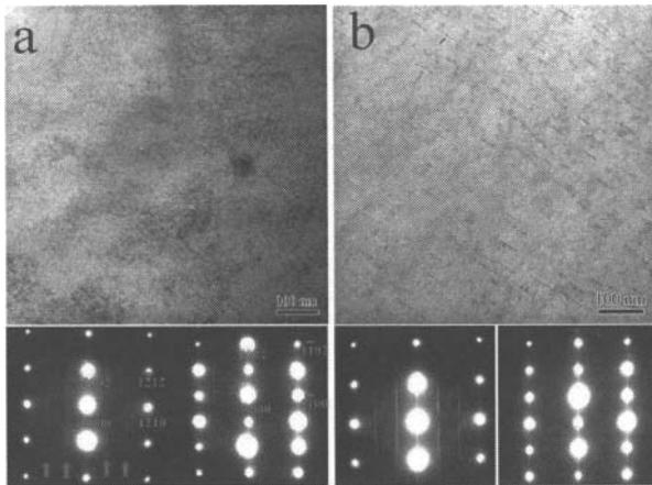
Figure 4 TEM bright field images of the Mg-0.5Ca-1Al aged alloy taken from the  $[10\bar{1}0]$  and corresponding SAED pattern of the  $[10\bar{1}0]$  and  $[11\bar{2}0]$  directions. (a) Peak aged at 200 °C for 4h (b) Over aged at 200 °C for 200h.
