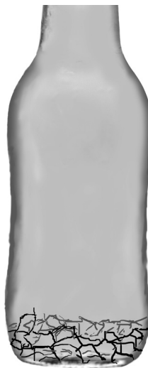
Figure 4.18. Water Hammer Failure in Glass Bottle
