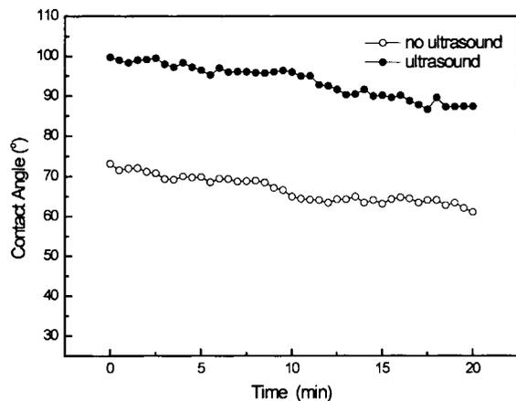
Figure 7. Curves of contact angles vs. time during wetting process of KF-AlF<sub>3</sub> melts (5 wt.% Al<sub>2</sub>O<sub>3</sub>, CR=1.3) on SMH cathode samples with ultrasound at 750 °C
