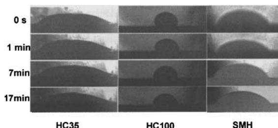
Figure 3. Photographs of KF-AlF<sub>3</sub> melts (3 wt.% Al<sub>2</sub>O<sub>3</sub>, CR=1.22) wetting on the three cathode samples at 750 °C
