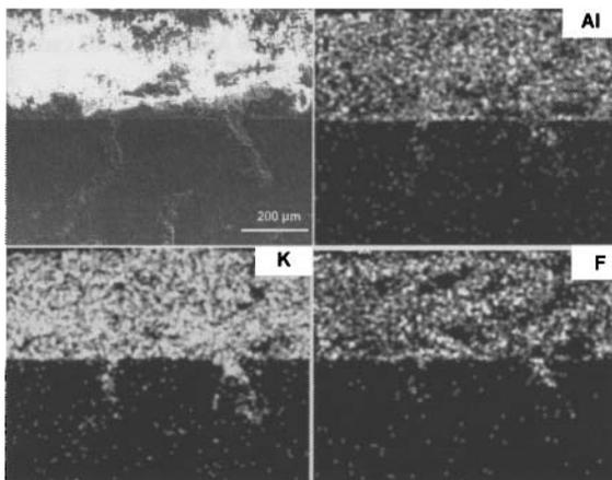
Figure 8. SEM image and EDS analysis on cross-sections at the melt-graphite interface after wetting tests (5 wt. %  $\text{Al}_2\text{O}_3$ , CR=1.5) on SMH cathode material at 750 °C
