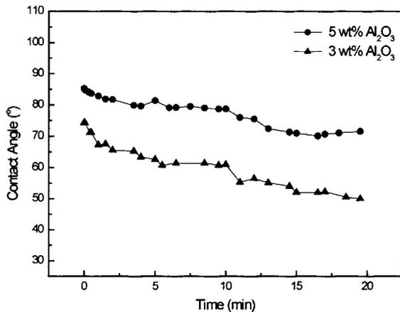
Figure 5. Curves of contact angles vs. time for different Al<sub>2</sub>O<sub>3</sub> contents in KF-AlF<sub>3</sub> melts wetting on SMH cathode material at 750 °C (CR = 1.22).
