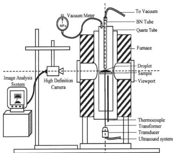
Figure 1. Schematic drawing of experimental set-up for sessile drop method.
