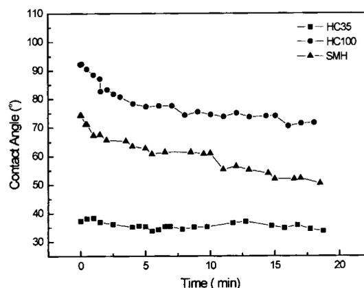
Figure 4. Curves of contact angles vs. time during wetting process of KF-AlF<sub>3</sub> melts (3 wt.% Al<sub>2</sub>O<sub>3</sub>, CR=1.22) on graphitic and graphite cathodes at 750 °C.
