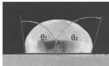
Figure 2. Scheme drawing of wetting angle calculation.
