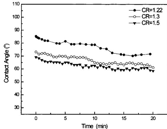
Figure 6. Curves of contact angles vs. time during wetting of KF-AlF<sub>3</sub> melts with various CR (5 wt.% Al<sub>2</sub>O<sub>3</sub>) on SMH cathode material at 750 °C
