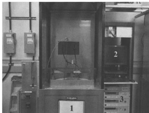
Figure 1. Electrolysis experimental setup with (1) oven and fume hood, (2) data acquisition and (3) power supply.
