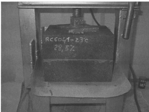
Figure 8: Gluing bench with two carbon slabs glued with a joint. Pressure is applied at the centre of the assembly.
