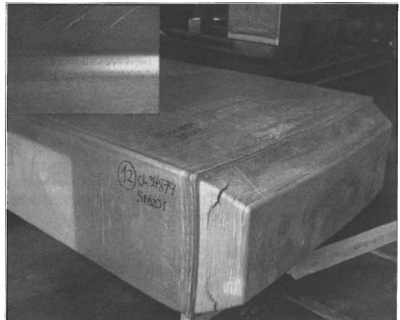
Figure 8. Flexible mould rolling slab; 600x1600mm, AA5182, Casting speed 60mm/min.
