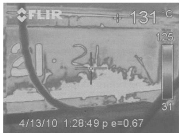
Figure 1: top is a FLIR image of a launder showing metal reaching shell (hot spot); bottom is a FLIR image of launder where the metal eventually enlarged the hot spot and ran into the bottom of the shell.
