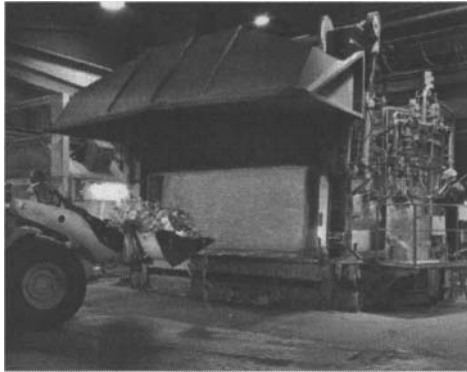
Figure 10. 28-tonne reverberatory melting furnace at Sapa Heat Transfer operated with four Low-temperature Oxyfuel burners since year 2005.
