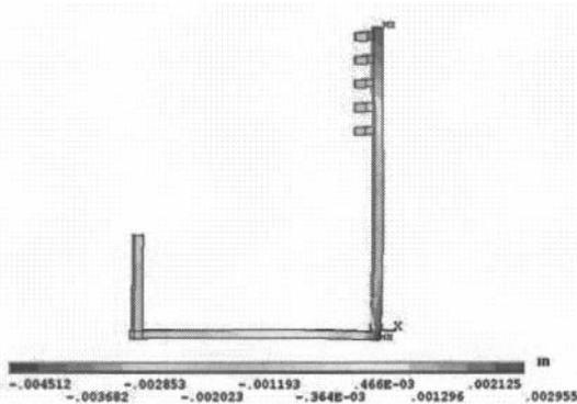
Fig.10. Y-displacement with two fixed brackets on round-end busbar
