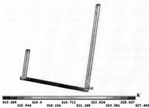
Fig.3. Temperature of cast-busbar
