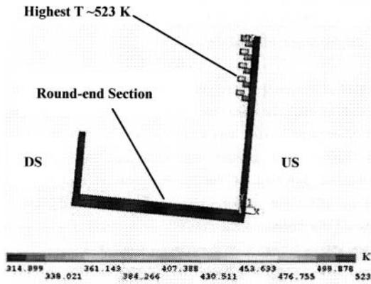
Fig.2. Temperature of the whole branch
