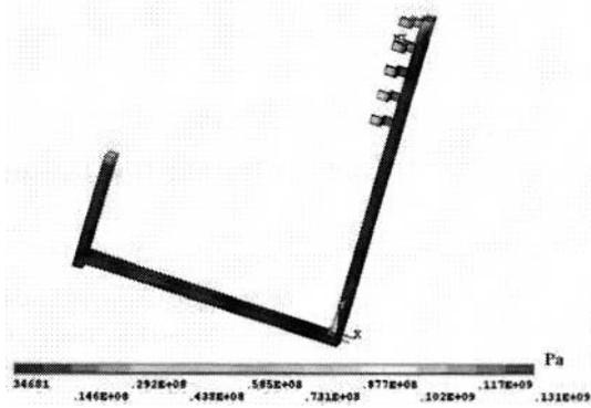
Fig.5. Busbar stress with only thermal effect
