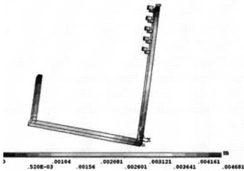
Fig.4. Busbar displacement with only thermoelectric effect
