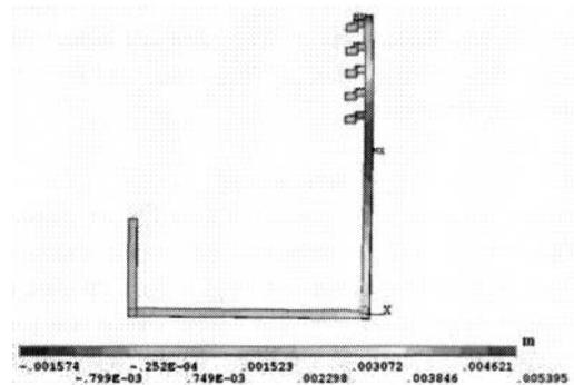
Fig.6. X-displacement of the busbar
