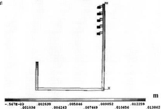
Fig.7. Y-displacement of the busbar
