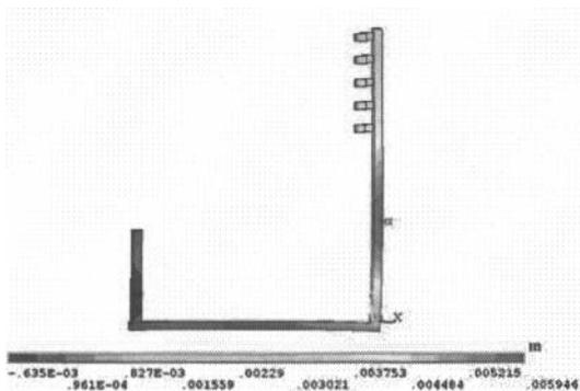
Fig.9. X-displacement with two fixed brackets on round-end busbar
