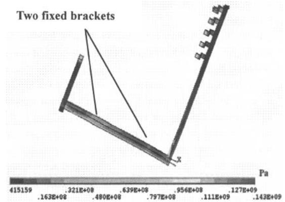
Fig.11. Busbar stress with two fixed brackets on round-end busbar
