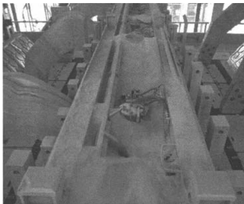
Figure 4 : Photo of pot with dusting. Dust is accumulating around the inlet to the pot hopper, but also around the ALF3 fill point.
