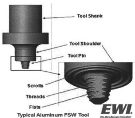
Figure 1. Friction Stir Weld tool
