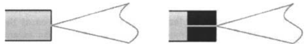
Figure 3. Sketch of the experimental setup: orifice nozzle ( d = 10^{-3} \text{ m} ) left and pipe nozzle ( d = 10^{-3} \text{ m} ) right hand side
